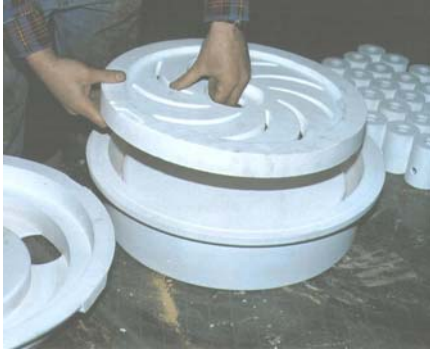
Fig 1: The cope and drag portions could be moulded of solid ceramic with the core being inserted before or after curing
