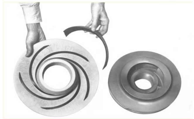
Fig 3: expendable wax vanes which are left in place for subsequent meltout in curing
